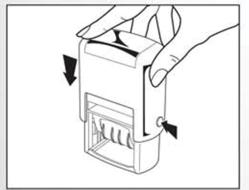
Press the Printy 4750's handle downward while pressing in the red side locking buttons until there is an audible click, locking the handle in place.
