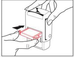
2. With the handle locked in place, slide the new ink cartridge in with the inked foam facing downward, making sure to utilize the new grip tabs to prevent inky fingers and ensure secure handling.
