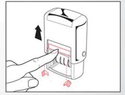
3. Push the ink cartridge all the way in until the grip tabs pop off and the cartridge clicks into place. Next, gently depress the handle to release the side locking buttons. Your Printy 4750 is ready to use.
